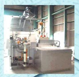
Aluminan melting and holding furnace Sectric immersed-type (SHE series)
